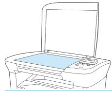
CAUTION: Do not use abrasives, acetone, benzene, ammonia, ethyl alcohol, or carbon tetrachloride on any part of the device; these can damage the device. Do not place liquids directly on the glass. They might seep under it and damage the device.
