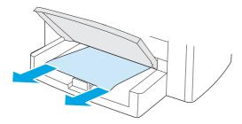
3. If no media is visible, open the print-cartridge door, remove the print cartridge, and then carefully pull the media up and out of the device.
