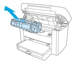
3. Remove the new print cartridge from its packaging, remove the cover from the print cartridge, and then pull the tab straight out to remove the sealing tape.
