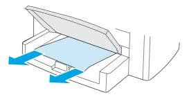
2. Open tray 1 and pull any visible jammed media out of the device.
