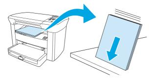
6. Maintaining the same orientation, place the stack of media in the input tray again. The printed side should be facing down with the top edge feeding into the device first.
