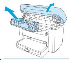
**CAUTION:** To prevent damage to the print cartridge, minimize its exposure to direct light.
