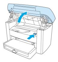
2. Grasp the handle on the print cartridge and then pull the cartridge straight out to remove it. See the recycling information inside the print cartridge box.
