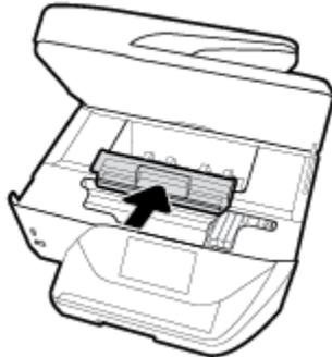
4. If the problem is not resolved, check the print carriage area inside the printer.
