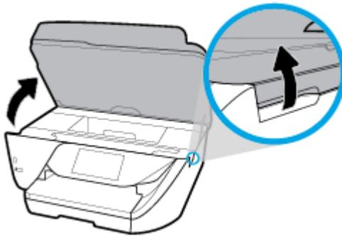
3. Check the paper path inside the printer.
