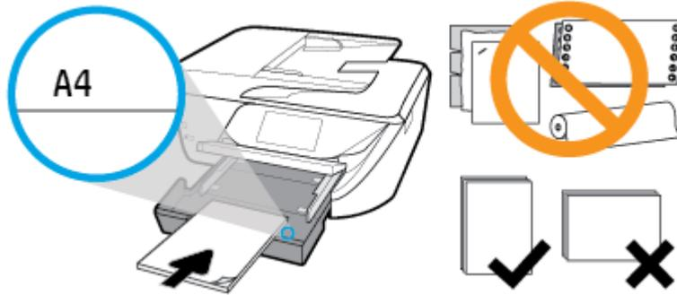
Ensure that the stack of paper is aligned with the appropriate paper size lines on the bottom of the input tray, and does not exceed the stack height marking on the side of the tray.
