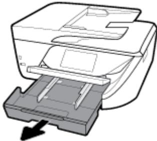
3. Press down the buttons on both sides of the input tray, and pull to remove the input tray.
