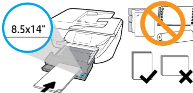
Make sure the stack of paper is aligned with the appropriate paper size lines on the front of the tray. Besides, make sure the stack of paper does not exceed the stack height marking on the edge of the tray.
