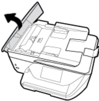
2. Lift the tab located on the front edge of the document feeder.
