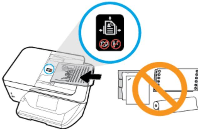
3. Slide the paper-width guides inward until they stop at the left and right edges of the paper.
