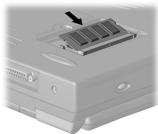
Installing the Memory Expansion Module
