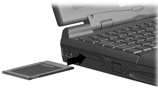
Inserting a PC Card
