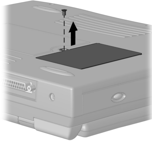
Removing the Screw
