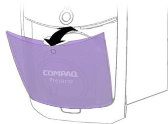
4. While the lower bezel is open, put your fingers in the finger holes under the upper bezel (marked with arrows on the computer). Then pull the upper bezel toward you to remove it.
