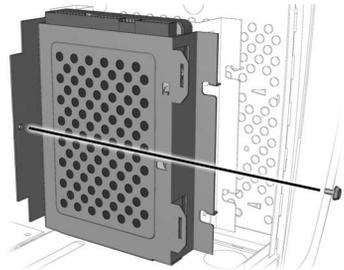
3. Mount the extra hard drive bracket tabs into the hooks on the hard drive bracket.
