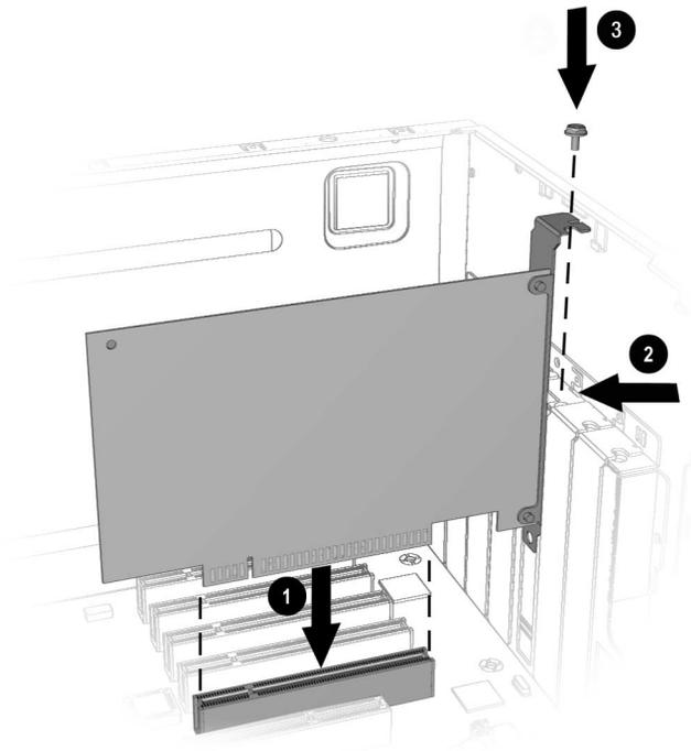
4. Place the slot screw **3** into the chassis slot and secure the expansion card to the chassis.
