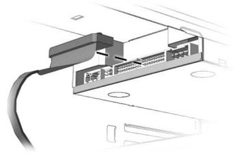
11. Connect the power cable to the drive.
