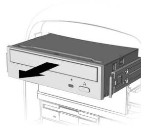
9. Remove the drive rails from each side of the drive and place the rails on the new drive. Slide the new drive back into the empty drive slot.
