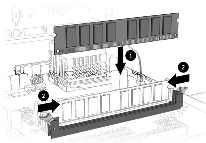
**Note:** Press gently to ensure the memory module is properly positioned.
