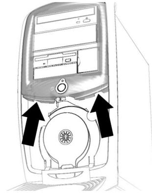
7. Push the plastic flaps on both sides of the drive inwards and pull towards you.
