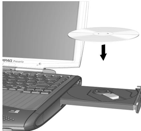
4. Push the tray back into the drive until the drive locks into place.
