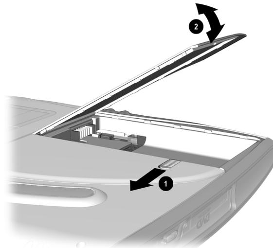
5. If a battery has been previously installed, use the tab on the battery to pull the battery out.
