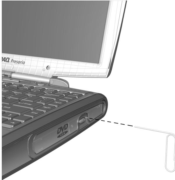
2. Insert a small rod or pin, such as a paper clip (approximately 1/16 inch in diameter and at least 3/8 inch in length) into the **Manual Eject Hole** and push firmly as shown in the figure above.
