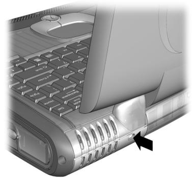
To remove the locking device, turn the locking device counter-clockwise 90 degrees and remove the device from the slot.
