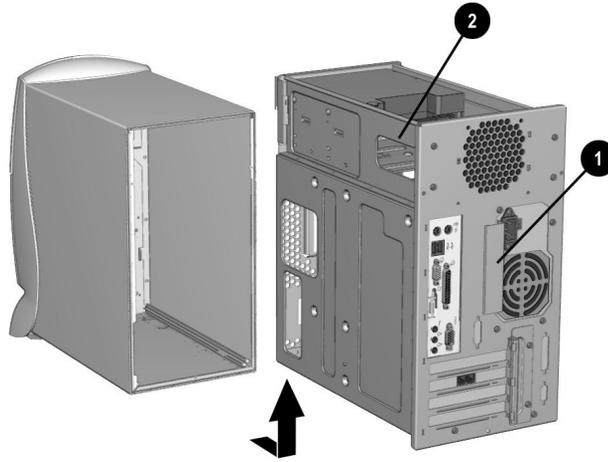
Removing the Chassis Cage
