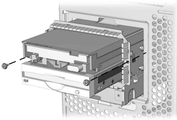
Removing the Drive Cage Retaining Screws
