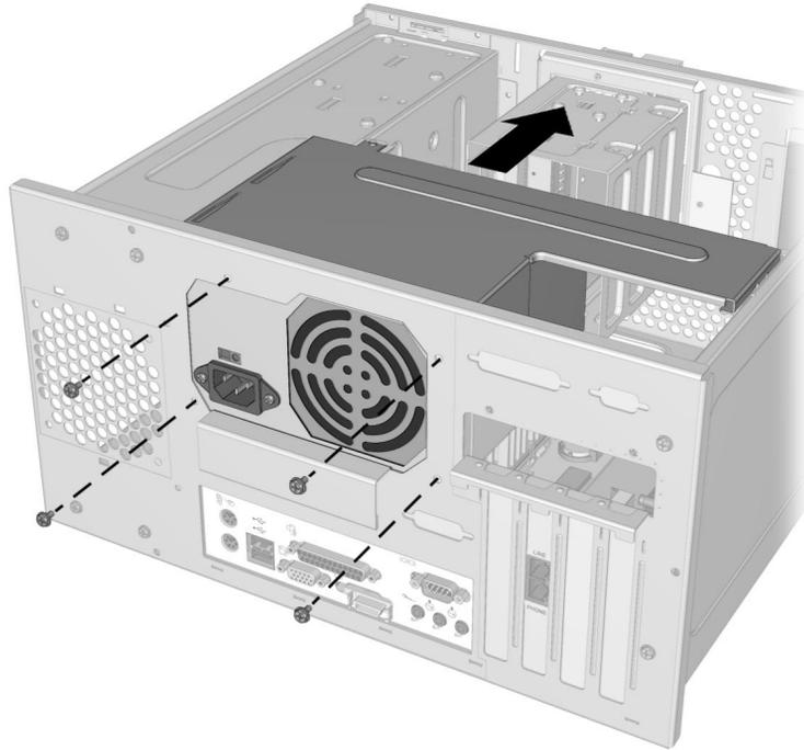
Removing the Power Supply Retaining Screws
