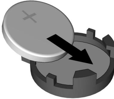
Inserting a Battery
