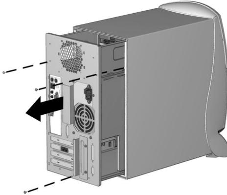
Removing the Cover Retaining Screws
