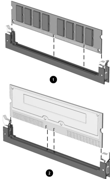
Inserting a Memory Module
