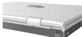
To remove the locking device, turn the locking device counter-clockwise 90 degrees and remove the device from the slot.
