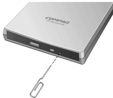
2. Insert a small rod or pin, such as a paper clip (approximately 1/16 inch in diameter and at least 3/8 inch in length) into the **Manual Eject Hole** and push firmly as shown in the figure above.
