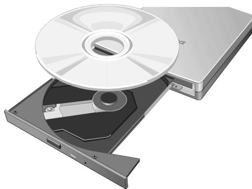
4. Push the tray back into the drive until the drive locks into place.
