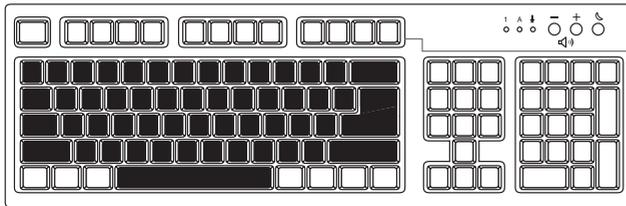
The alphanumeric keys are the main keys found on a standard typewriter.
