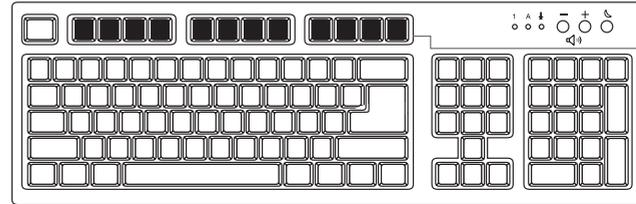
The function keys are the F1 through F12 keys located above the main keys. Pressing F1 displays a Help window for the software program being used. Pressing F3 displays a search window. F1 and F3 are available during normal operation. Other function key operations may depend on what software program you are using.
