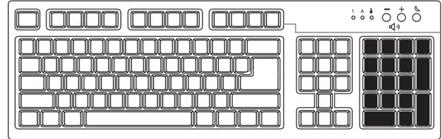
When the Num Lock LED (light-emitting diode) on the keyboard is on, the numeric keys are enabled to function similar to those found on a basic calculator. When the Num Lock LED on the keyboard is off, the numeric keys are directional keys used during games or to move the cursor. Press the Num Lock key to lock and unlock the numeric key functions.
