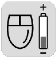
**Note:** *The Low Battery icon appears 5 times each hour until the batteries are changed. If you use a mouse pad, choose a light-colored one, not a dark one, to conserve battery power.*
