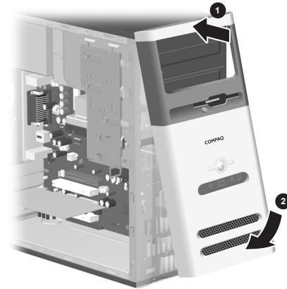
Removing the front bezel from the S series
