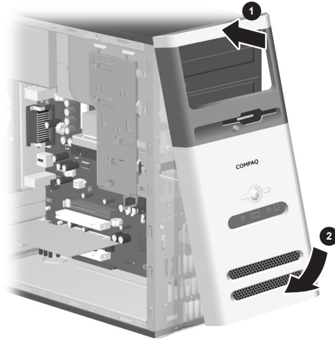
Replacing the front bezel on the S series
