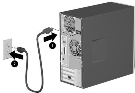
**reconnecting the power cable on the S0000/8000 (S0000 shown)**
