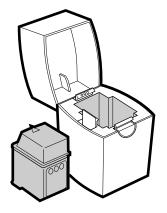
The optional Color Kit which includes a color print cartridge and a print cartridge storage container, provides color output printing capability from an HP DeskJet 600 printer. The printer comes from the factory as color capable, it does not require any modifications. Color features, however, need to be turned on in the printer driver dialog box in MS Windows. For more information, refer to the HP DeskJet 600 printer user documentation or to the information included with the Color Kit.
