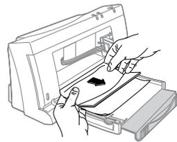
7. After clearing the paper jam, close the paper separator.
