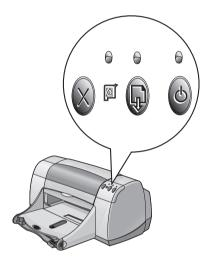
Power Button and Light – Use the Power Button to turn the printer on and off. When the green light above the Power Button flashes, printing is in progress.
