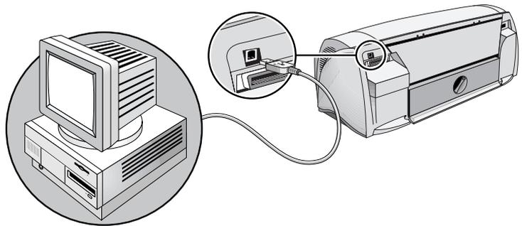
The latest personal computers have USB ports that can be directly connected to the printer's USB port. After connecting the USB cable, the **New Hardware Found Wizard** should appear. If it does not, your computer is probably not configured to use USB. Use a parallel cable instead to connect the printer to your computer.
