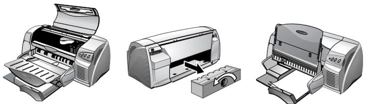
Note: To clear the printer of any jammed paper, open the access cover and pull the paper towards you. If you cannot reach the jammed paper, turn the panel
