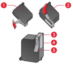
1. black print cartridge 2. tri-color print cartridge 3. ink nozzles 4. copper contacts—do not touch or remove the copper contacts 5. protective vinyl tape—remove only the protective vinyl tape
