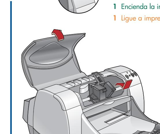
Step 7: Install print cartridges, then calibration page prints
