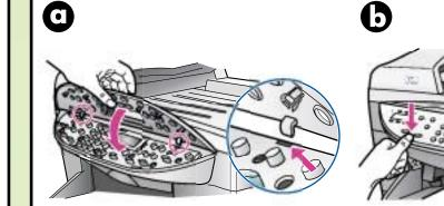
Insert the two tabs of the cover into the top slots on the unit.
