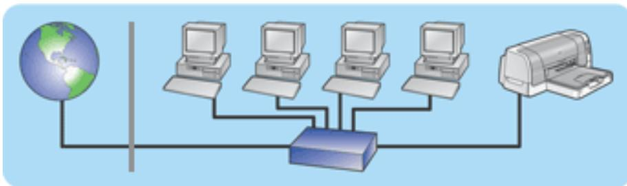
This example looks similar to the first example. However, in this example, the network devices are connected to a [hub](#), rather than a [router](#). The hub is directly connected to the Internet.
