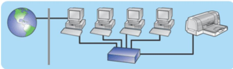
In this example, the network devices are connected to a [hub](#). A computer on the network acts as the [gateway](#) between the network and the Internet. The gateway computer uses [Windows Internet Connection Sharing \(ICS\)](#) to manage the network connections and provide Internet access to the other devices.
