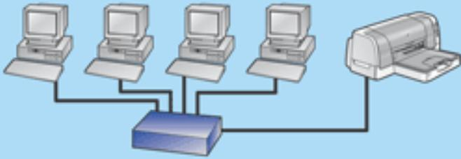
In this example, the network devices are connected to a [hub](#). Devices use [AutoIP](#) to obtain [IP addresses](#).
