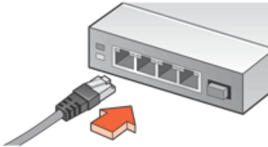
4. Connect the [ethernet cable](#) to the ethernet port on the back of the printer.
