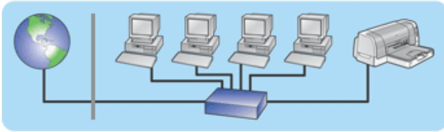
In this example, a [router](#) manages the network connections and acts as a [gateway](#) between the network and the Internet.
