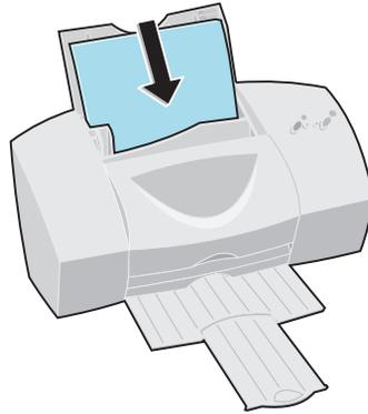
Squeeze the release tab and the paper guide together, and slide the paper guide to the edge of the photo paper.
