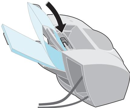
**e** Squeeze the release tab and the paper guide together and slide the paper guide to the edge of the banner.
