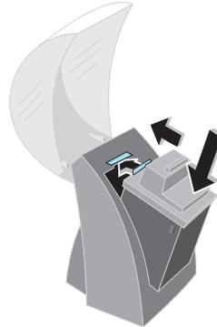
**e** Remove the sticker and tape covering the gold contact area of the photo print cartridge.
