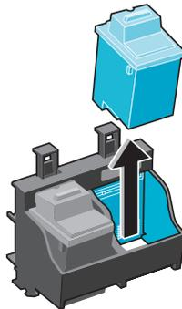
**d** Store the black cartridge temporarily in the print cartridge storage unit that came with your photo cartridge.
