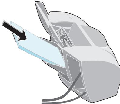
**d** Insert the unattached edge of the first page into the automatic feeder.
