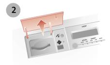
Lift up on the door to reveal the card slot.
