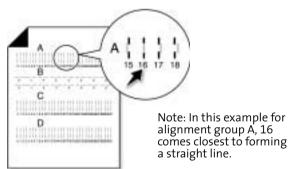
Using the same **Up**, **Down** and **Enter** buttons used in step 4, change the value for the letter displayed on the printer LCD, and then press Enter to select it. The next alignment letter will be shown until you have set all the alignment values for the page.
