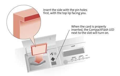
**WARNING**: Never remove the memory card when the CompactFlash light is flashing, or you could damage the card.
