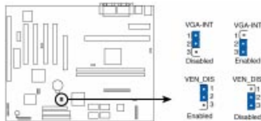
Figure 5-17: VGA Interrupt Jumper Settings
