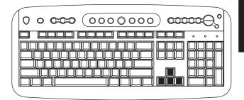
The arrow keys are controls for up, down, right, and left. You can use these keys instead of the mouse to move the cursor for navigation in a Web site, in a document, or in a game.
