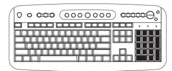
When the Num Lock LED (light-emitting diode) on the keyboard is on, the numeric keys are the number keys and arithmetic functions found on a basic calculator. When the Num Lock LED on the keyboard is off, the numeric keys are directional keys used during games or to move the cursor. Press the *Num Lock* key to lock and unlock the numeric key functions.
