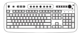
The special buttons are at the top of the keyboard. (Some models have some of these special buttons on the left side of the main keys.) These buttons operate a CD-ROM or DVD-ROM player, connect you to the Internet, or provide quick access to specific functions. To find out what each special button does, see "Buttons" on page 16.
