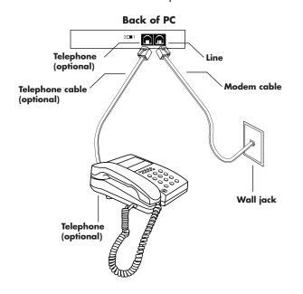
You can also connect a telephone to the other connector on the modem (optional). By connecting a telephone to the modem, you can make regular (voice) telephone calls when you are not using the modem — even if the computer is turned off.
