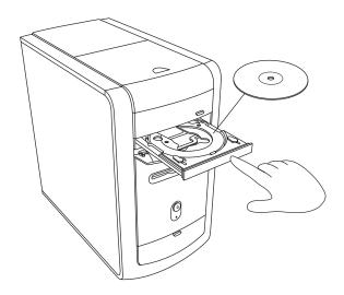
5 Close the disc tray by gently pushing the tray into the computer. You can also close the tray by clicking the close/open button on the control panel for the program (such as MusicMatch Jukebox or Windows Media Player) that controls the drive.
