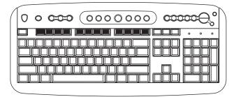
The function keys are the F1 through F12 keys located above the main keys. Pressing F1 displays a Help window for the software program being used. Pressing F3 displays a search window. F1 and F3 are available at all times. Other function key operations may depend on what software program you are using.
