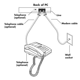
You can also connect a telephone to the other connector on the modem (optional). By connecting a telephone to the modem, you can make regular (voice) telephone calls when you are not using the modem — even if the computer is turned off.
