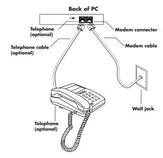
You can also connect a telephone to the other connector on the modem (optional). By connecting a telephone to the modem, you can make regular (voice) telephone calls when you are not using the modem — even if the PC is turned off.
