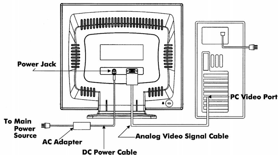
4. Plug the analog video signal cable into the Analog Video Input port on the back of the monitor (as shown above).
