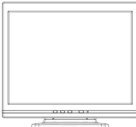
Use the power button located at the lower middle of the front panel of your monitor to turn on and off the monitor.
