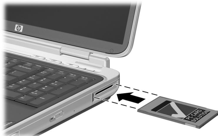
*Inserting a PC Card*
