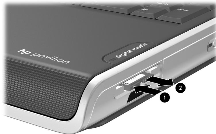
*Releasing and removing a digital media card*
