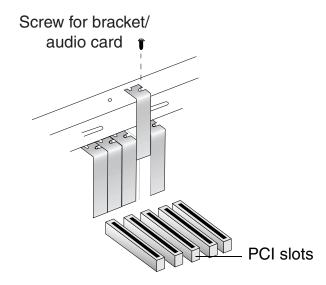
**4** Remove the bracket of an unused PCI slot if you do not already have an audio card installed, or remove the existing audio card. Put the screw aside.
