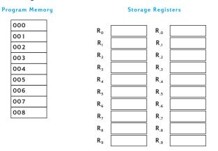
As you key in a 310th instruction, storage register  $R_{0.9}$  is automatically converted into seven new lines of program memory. The instruction you key in is stored in program line 310, and the instruction GTO 000 is automatically stored in program lines 311 through 316.
