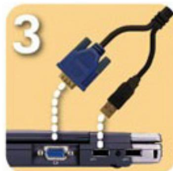
Connect the blue end of the video cable to the PC; optionally, to have the remote control function as a mouse, connect the USB connector to the PC.
