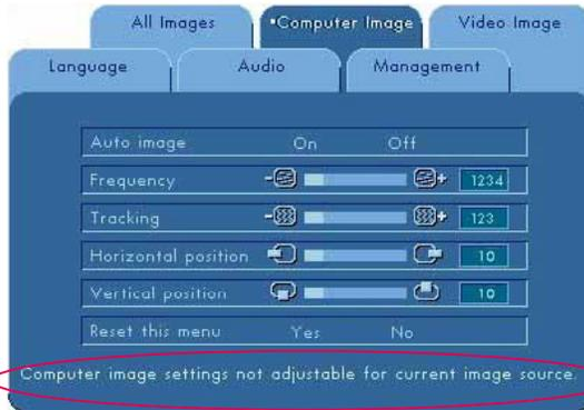
**NOTE:** This message is displayed when an image source other than computer VGA is selected via the **Source** button or the auto detection function.
