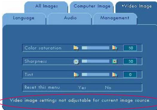
**NOTE:** This message is displayed when these settings cannot be adjusted for the image source selected via the **Source** button or the auto detection function (i.e. computer VGA or 480p).
