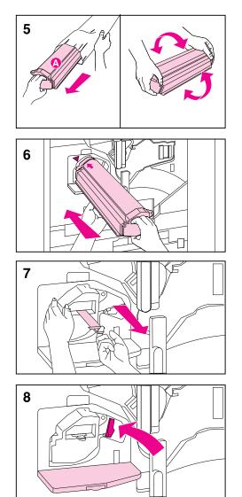
**5** Remove the toner cartridge that matches the color of the sticker in the carousel slot from its packaging and gently rock the cartridge several times to distribute the toner.
