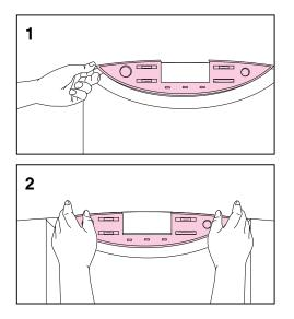
Replace the printer control panel overlay with the one included for your language, if applicable. Then configure the printer control panel to show printer messages in your language.
