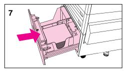
5 Load media into the tray up to the media-fill mark. For example, up to 2,000 sheets of 20 lb (75 g/m<sup>2</sup>) bond paper will fit in the tray. For information on loading and orienting media, see the online user's guide or the quick reference guide.
