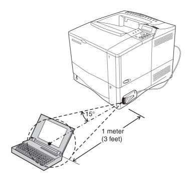
Figure 5 Alignment of Devices Used for Printing
