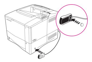
Figure 3 Attaching the Velcro Fasteners
