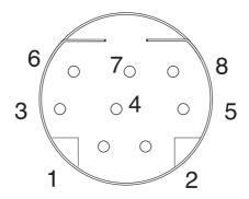
Figure 6 Eight-Position Mini-DIN Connector
