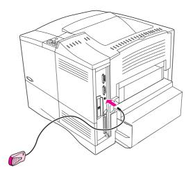
Figure 2 IR Port on a HP LaserJet Printer
