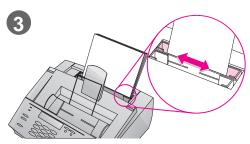
You can load up to 100 sheets of 20 lb  $(75 \text{ g/m}^2)$  paper into the paper input bin. The HP LaserJet 3150 product prints, copies, and prints received faxes using media from the paper input bin (or the single-sheet input slot).
