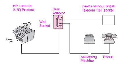
Before you begin, plug a dual adaptor (not included) into the cord for the HP LaserJet product. Then, if you are not connecting one (or more) of the devices shown, just cross it out. Finally, in the manner indicated, connect the devices you do have. See the next page for step-by-step instructions.
