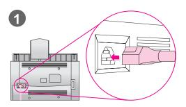
The HP LaserJet 3150 product does not have a power switch. It turns on when the power cord is connected.
