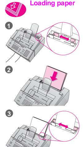
You can load up to 100 sheets of 20 lb  $(75 \text{ g/m}^2)$  paper into the paper input bin. The HP LaserJet 3150 product prints, copies, and prints received faxes using media from the paper input bin (or the single-sheet input slot).
