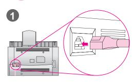
The HP LaserJet 3150 product does not have a power switch. It turns on when the power cord is connected.
