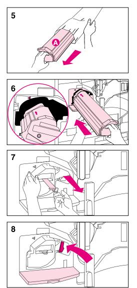
5 Remove the toner cartridge that matches the color of the sticker in the carousel slot from its packaging.
