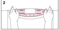
Replace the printer control panel overlay with the one included for your language, if applicable. Then configure the printer control panel to show printer messages in your language.
