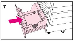
5 Load media into the tray up to the media-fill mark. For example, up to 2,000 sheets of 20 lb. (75 g/m<sup>2</sup>) bond paper will fit in the tray. For information on loading and orienting media, see the online user guide or the quick reference guide.
