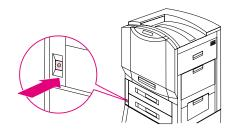
1 Hold down SELECT while turning the printer on (power button in). SELECT LANGUAGE (in English) appears on the printer control panel display for approximately one second. Once the printer has restarted, LANGUAGE = ENGLISH will appear on the display.
