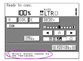
Figure 57 Toner cartridge message - \*\* (COLOR) TONER NEEDS TO BE REPLACED
