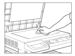
Figure 64 Cleaning the copy module glass
