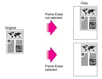
Figure 30 Image without and with the dark border erased
