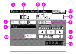
Figure 10 Touch panel display—Basic Features screen
