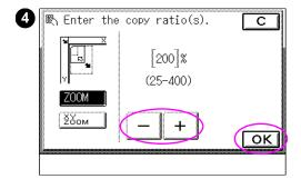
4 Specify the copy ratio (%), using the numeric keys on the control panel or press - or + in the touch panel display. After confirming the settings, press OK, and then press START on the copy module control panel to begin the copy job.
