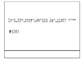
Figure 63 Service-call message on the touch panel display
