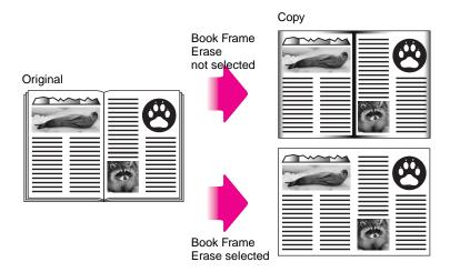
Figure 32 Image with center line and dark border erased
