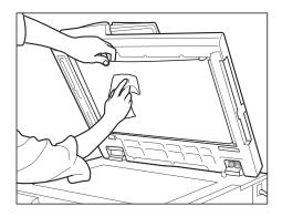
Figure 66 Cleaning the feeding belt
