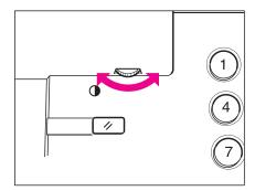
Figure 9 Control panel display contrast adjustment
