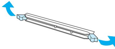
Check that the locks on each side of the DIMM SLOT 0 are opened (outward).
