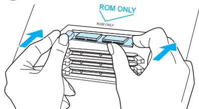
Press the DIMM straight into the slot (press **firmly**). Make sure the locks on each side of the DIMM slot snap inward into place.
