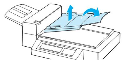
Lift the input tray up to lock it into place. For longer paper, flip the tray extension out as shown.
