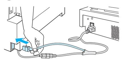
Plug the long end of the Y power cord into the printer.
