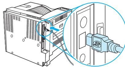
Plug the other end of the Copy Connect cable into the Copy Connect EIO Board. (The HP logo facing as shown.)
