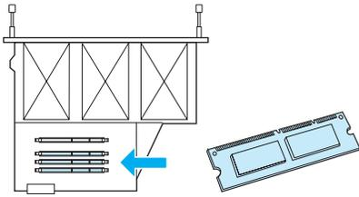
Align the notches on the DIMM with the keys in the first open DIMM slot. Check that the locks on each side of the DIMM slot are opened (outward). Press the DIMM straight into the slot (press **firmly**).
