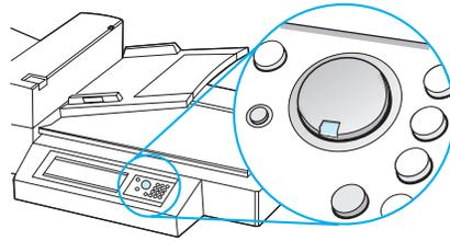
The green LED lights up on the **START** button to show that the HP Digital Copy is ready to copy.
