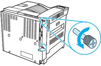
Loosen the two captive thumbscrews on the left rear of the printer.
