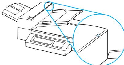
A green LED lights up on the automatic document feeder cover to show that you have properly inserted the documents into the feeder.
