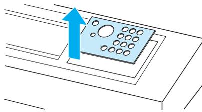
If necessary, remove the English control panel overlay. To remove the control panel overlay, insert a screwdriver into the slot on the left side of the overlay.
