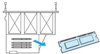
Identify SLOT 0 (labeled ROM ONLY). If another DIMM occupies this slot, snap the locks on each side of the DIMM outward and pull it out. **CAUTION!** Use antistatic protection for steps 15-23.
