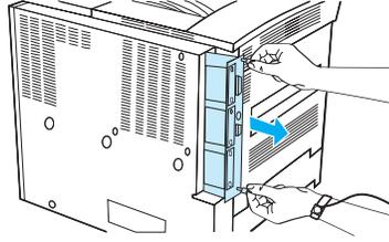
Grasp the screws and pull the formatter board out of the printer. Place it on a flat, non-conductive surface.
