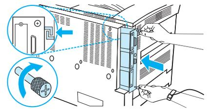
Slide the formatter board back into the printer and tighten the two screws. (Make sure the formatter board aligns with the guide tracks at the top of the printer.)
