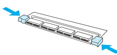
Make sure the locks on each side of the DIMM snap inward into place.
