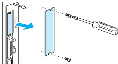
For the next two steps, use a screwdriver to remove the screws and covers from the EIO slots. Save the screws.
