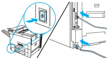
Plug in the power cord and connect all cables. Turn the printer on.
