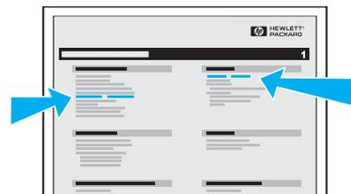
The total memory should be 48 MB or higher. **HP LaserJet 8000 Family:** the Firmware Datecode should end with 4.48 or higher. **HP LaserJet 8100 Family:** the Firmware Datecode should end with 5.44 or higher.
