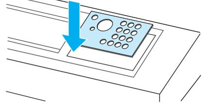
Press the overlay in place on the HP Digital Copy control panel until it clicks.
