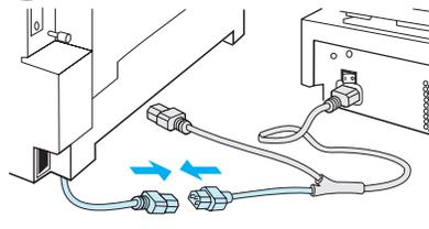
Unplug the power cord from the printer. Plug the power cord into the short end of the Y power cord.
