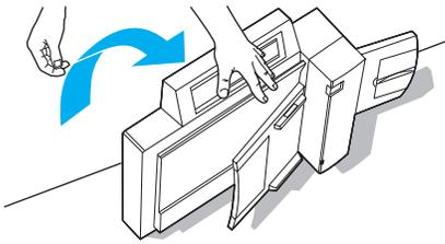
**CAUTION!** Ensure that the document cover does not swing backward and cause damage. Tip the copy module back.
