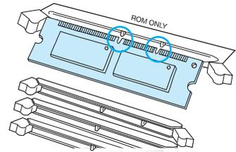
Remove the firmware upgrade DIMM from the antistatic package. Hold the DIMM with fingers against the side edges and thumbs against the top edge. **Align the notches on the DIMM with the keys in DIMM SLOT 0.**
