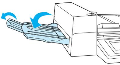
Pull the output bin down. For longer paper, flip the bin extension out as shown.
