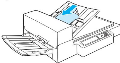
Load the original document face down into the automatic document feeder or place it on the flatbed of the HP Digital Copy. Select the desired number of copies.
