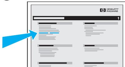
On the Configuration Page, check the Firmware Datecode located under the Printer Information box.
