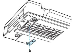
Rotate the shipping lock and reinsert it into the HP Digital Copy in the unlocked position (this shipping lock is necessary for future moves).
