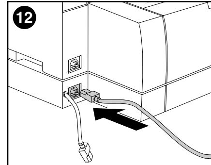
Plug the power cord from the back of the printer into the duplex printing accessory.
