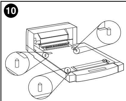
Use the guide pins on the duplex printing accessory to align the printer as you lower it onto the duplex printing accessory.
