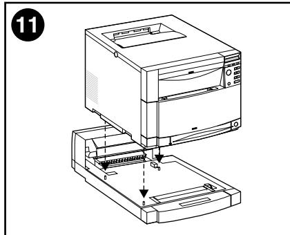
Gently lower the printer onto the duplex printing accessory. **CAUTION:** Avoid bending the guide pins while lowering the printer.
