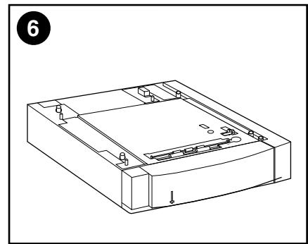
If you also are installing the optional 500-sheet paper feeder, install it now. For instructions, see the *500-Sheet Paper Feeder Installation Guide*.
