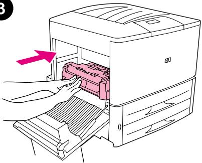
Using both hands, slide the duplexer into the printer until the unit locks into place.
