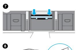
7 Snap both sides of the separation pad firmly into place.
