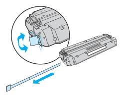
Remove the toner cartridge from the plastic bag. To remove the mylar tape, break the tab on the left and pull the tape completely out.
