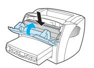
When toner is low, faded or light areas appear on the printed page. You might be able to temporarily improve print quality by redistributing the toner, which means that you might be able to finish the current print job before replacing the toner cartridge.
