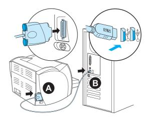
Plug the pod on the USB cable into the printer (A). Plug the USB cable into the PC (B).
