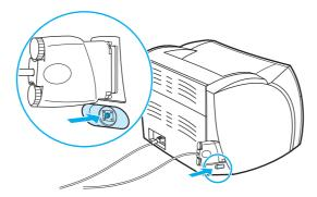
The engine test page prints as either a striped page or a solid black page. If the engine test page does not print, see <u>Status light patterns</u> for more information. If the engine test page prints as a white page, see <u>Missing graphics or text, or blank pages</u> for more information.
