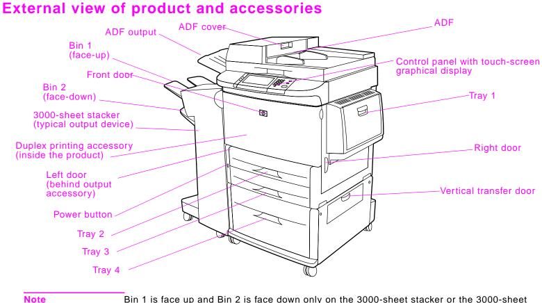
Bin 1 is face up and Bin 2 is face down only on the 3000-sheet stacker or the 3000-sheet stapler/stacker. If you choose the multifunction finisher as your output device, Bin 1 is both face up and face down, and Bin 2 is the booklet bin.
