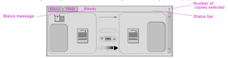
You navigate through the control panel menus using the touch-screen graphical display.
