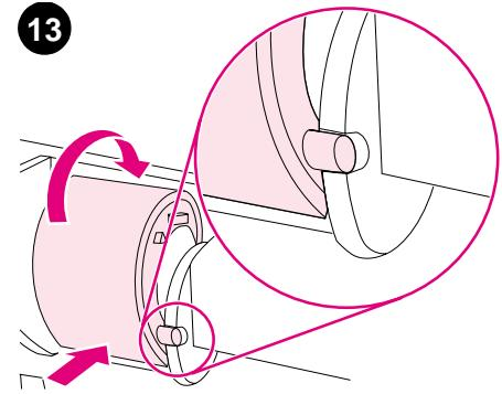
Place the new pickup roller onto the shaft. Align the pin that is located on each side at the bottom of the roller with the slot in the bracket located on each side of the opening. Slide the roller into the printer until the roller snaps into place.
