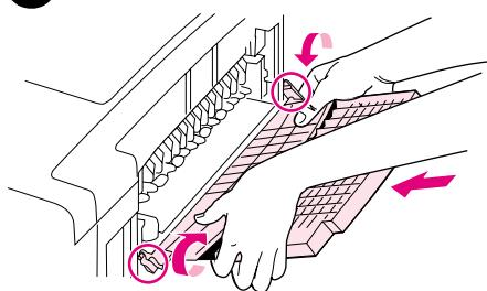
Install the rear output bin. Pull gently on the bin to make sure that the hinge pins are fully inserted.
