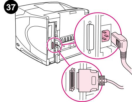
Connect the cables to the rear of the printer.
