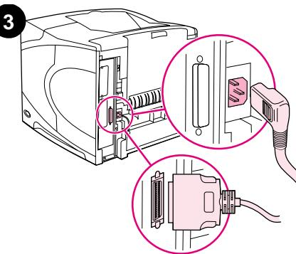
Disconnect all cables from the rear of the printer.
