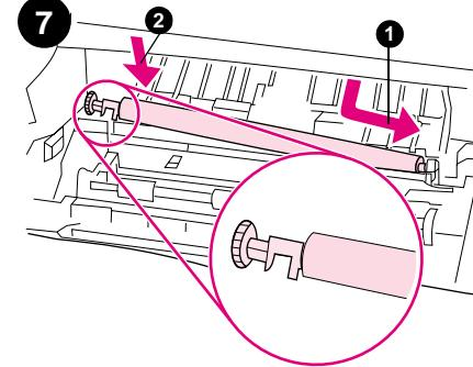
Make sure that the black collar on the left side is oriented properly, with the open end down. Install the new transfer roller by sliding the right side into place (1). Snap the left side (with the gear) into place (2).
