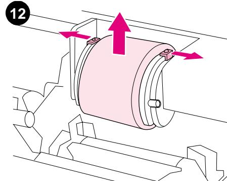
Release the roller by sliding apart the two latches located on each side at the top of the roller. Lift the roller out of the opening.
