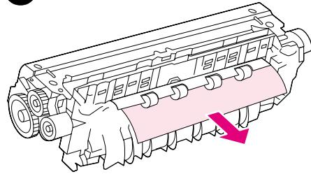
Remove all packing material from the new fuser.
