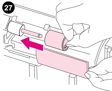
Slide the new feed roller onto the shaft.
