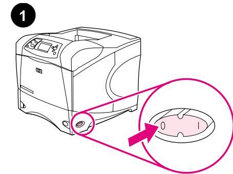
Turn the printer power off. **WARNING!** After you turn the printer power off, allow the fuser to cool for 30 minutes before proceeding.
