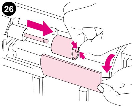
Pinch the blue latch that is on the side of the feed roller and slide the roller off the shaft.
