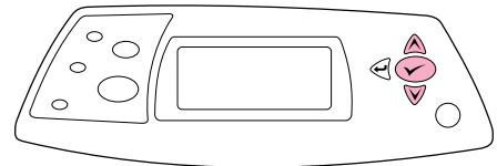
To verify that installation is complete, print a configuration page from the control panel. Press **✓** to open the printer menus. Press **▼** to select **INFORMATION**, and then press **✓**. Press **▼** to select **PRINT CONFIGURATION**, and then press **✓**.
