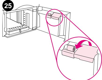
On the inside of the door, open the small cover next to the feed roller.
