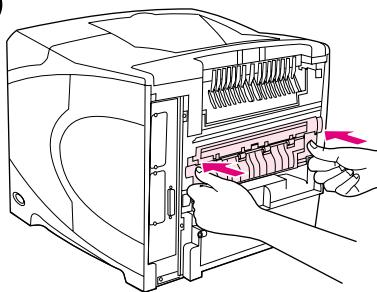
Push the new fuser firmly into the printer until the blue levers on both sides click into place.
