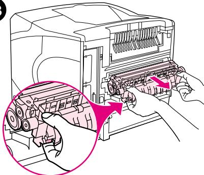
Firmly grasp each side of the fuser. Push the blue levers upward and pull the fuser straight out of the printer. **WARNING!** The fuser might be hot. Make sure that the printer has been turned off for 30 minutes before removing the fuser.
