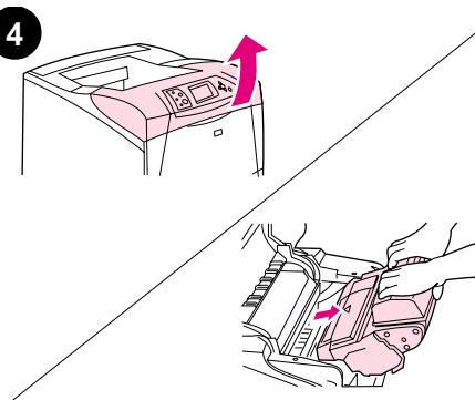
To replace the transfer roller: Turn the printer so that the front is facing you. Open the top cover and remove the print cartridge. Locate the transfer roller beneath the area from which the print cartridge was removed.
