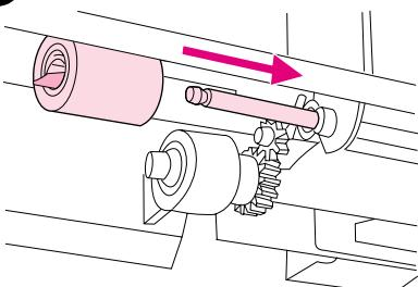
Slide a new feed roller onto the shaft and rotate the roller until it locks into place. **Note:** It is important that the roller locks into place.
