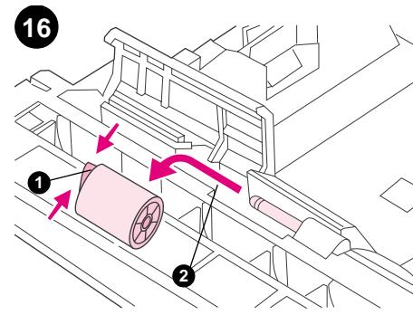
Pinch the blue latch that is on the left side of the feed roller (1). Slide the roller off the shaft (2).
