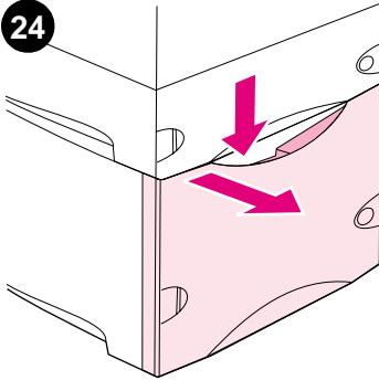
Push down on the release lever and open the door of the 1500-sheet feeder.
