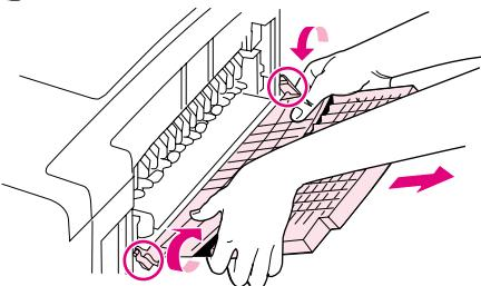
Remove the rear output bin and extension by bending the middle of the bin down and releasing the two hinge pins.
