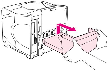
Turn the printer so that its rear cover faces you. Lift and pull to remove the optional duplexer, if it is installed.
