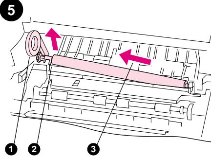
Use the plastic transfer-roller tool (1) to lift the left end of the metal shaft upward (2). Slide the transfer roller to the left and remove it (3).
