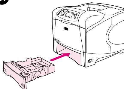
Insert tray 2. If no optional trays are installed, go to step 31.
