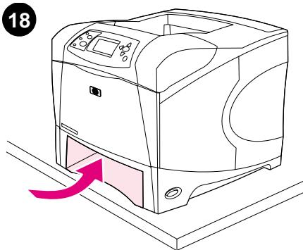
Move the front of the printer to the edge of the table top for better access to the feed roller that is located inside the printer. **WARNING!** Do not allow the front of the printer to extend beyond the edge of the table. The printer can become unbalanced and fall, causing damage or injury.
