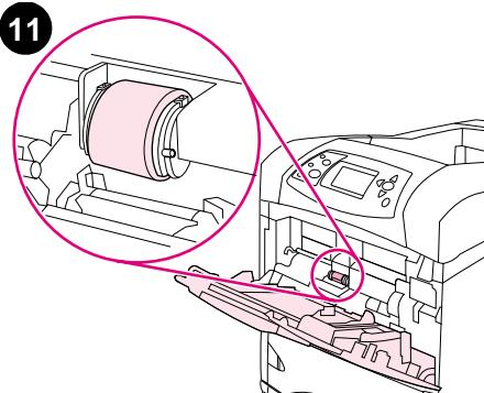
Locate the pickup roller at the center of tray 1.
