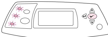
To finish the installation: Turn the printer power on while holding down **✓** for several seconds, until all three control panel lights turn on and remain on. Press **▲** until the **NEW MAINTENANCE KIT** message appears on the display, and then press **✓**.
