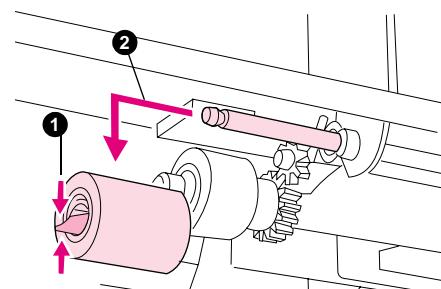
Pinch the blue latch on the left side of the feed roller (1). Slide the roller off the shaft (2). You might need to rotate the roller in order to pinch the latch.
