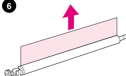
Put on the gloves and remove the protective sheet from the new transfer roller. **CAUTION:** Do not touch the new transfer roller with bare hands. Skin oils on the roller can cause print-quality problems.
