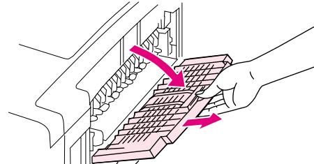
To replace the fuser: Open the rear output bin and pull the extension outward until it stops.
