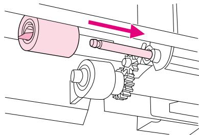
Slide a new feed roller onto the shaft and rotate the roller until it locks into place. **Note:** It is important that the roller locks into place.
