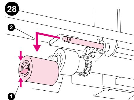
Locate the roller at the top-center inside the 1500-sheet feeder. Pinch the blue latch that is on the left side of the roller (1). Slide the roller off the shaft (2). **Note:** It might be necessary to rotate the roller in order to pinch the latch.
