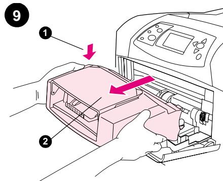
To replace the tray-1 pickup roller: If an optional envelope feeder is installed, remove it by pressing the envelope-feeder release button (1) and pulling outward on the envelope feeder (2).
