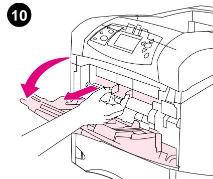
If an optional envelope feeder is not installed, open tray 1 and remove the envelope-entrance cover.
