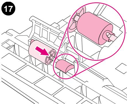
Slide a new feed roller onto the shaft. **Note:** It is important that this roller locks into place. If it does not, make sure that the roller is properly oriented, and that the round, black spacer next to the roller is properly positioned around the pin in the shaft.
