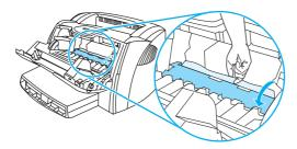
**6** When you have removed the jammed media, replace the print cartridge, and close the print cartridge door and the straight-through output door.
