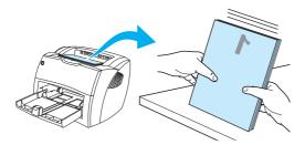
8 Place the pages from side one back in the input tray. Side one should be facing down with the bottom edge feeding into the printer first.
