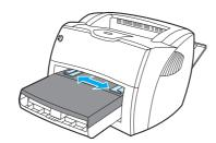
3 Place the envelope with the side to be printed facing up and the top edge along the left media guide.
