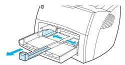
3 Place the envelopes with the side to be printed facing up and the top edge along the left media guide. Stack up to 30 envelopes.
