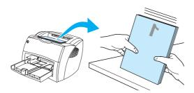
**8** Place the stack back in the input tray. Side one should be facing down with the bottom edge feeding into the printer first. Replace the priority input tray.
