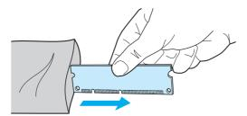
5 Position the DIMM chip in front of the slot located inside the I/O door. The gold contacts should be pointing toward the printer and the cutouts should be at the top and bottom.
