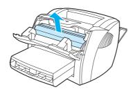
4 With both hands, grasp the side of the media that is most visible (this includes the middle), and carefully pull it free from the printer.
