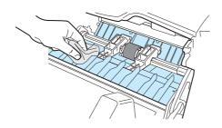
**3** Replace the print cartridge, and close the print cartridge door.
