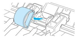
6 Position the new or cleaned part in the slot of the previous pickup roller. See <u>Cleaning the pickup roller</u> for instructions.
