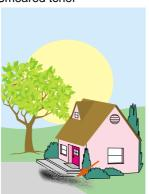
This occurs because the wrong type is set for the media or because the inks used on a preprinted form melt under the temperature of the fuser.
