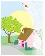
This can be caused by rough media or by using the wrong media type.
