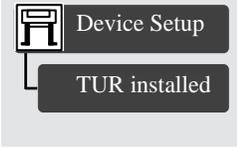
**1.** Using the front panel, select the Printer Setup menu, then “Device Setup”, then “TUR installed”, and change the value of this option from **No** to **Yes**.
