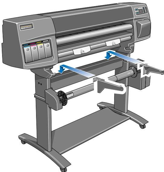
**33.** Slide each of the deflector supports sideways until the T-piece on top of the support is fully inserted into the gap between the cross brace and the printer leg. The deflector support should now be touching the take-up reel assembly.
