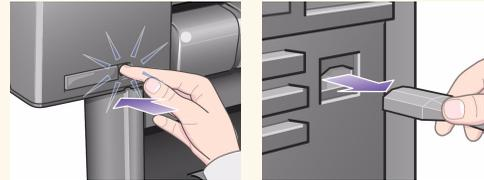
2. Carefully remove the plastic cover from the left-hand back of the printer by unclipping it. This cover gives access to the two slots for an Accessory card and a LAN card.
