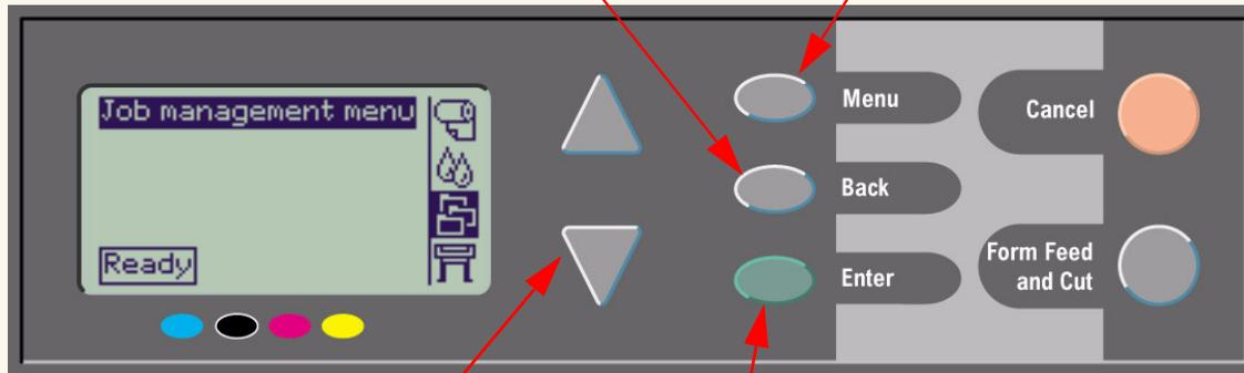
Press the **Up** ▲ and **Down** ▼ keys to scroll up and down through the menus or menu options.
