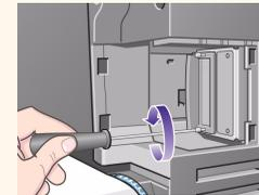
5. When you have inserted the card, screw it into place, using its two screws (at the top and bottom of the card). Again, this can be done with a screwdriver or manually.
