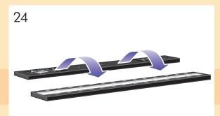
Turn the pressure platen over to expose the white background plate.
