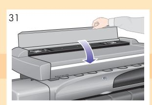
With the platen firmly locked into place; close the scanner cover.
