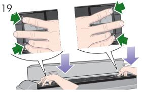
Position your fingers in the 4 lock slots (2 at each end of the platen indicated by the green arrows above), and press down (blue arrows).
