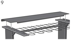
Connect the rear table: this is fitted by locating the 4 guide pins on the rear of the table into the rubber framed holes on the top bar.
