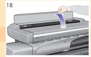
Open the scanner cover to expose the scan area.
