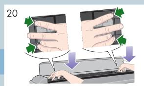
Position your fingers in the four lock slots (two at each end of the platen indicated by the green arrows above), and press down (blue arrows).
