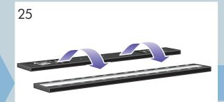
Turn the pressure platen over to expose the white background plate.
