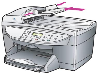
Slide the automatic document feeder (ADF) tray extension into the top of the copier. Match the gray tabs with the black slots.
